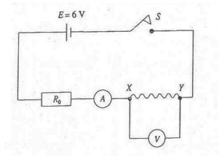
Figure shows a simple experimental arrangement to find the resistivity of a nichrome wire XY. Resistance of the wire is found to be in the order of  $100\Omega$ . A is a micro ammeter having a full scale deflection of 100  $\mu$ A. E is a 6V cell with negligible internal resistance.  $R_0$  is a fixed resistor, and V is a voltmeter. (Both A and V can be considered as ideal instruments).
